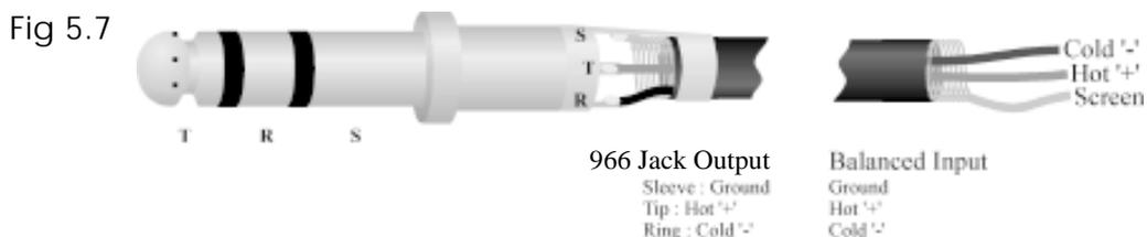
Connection to unbalanced inputs may be done by connecting the tip to the signal input, and the ring to the input shield. The FCS 966 shield may or may not be connected to the equipment shield at the equipment end.
