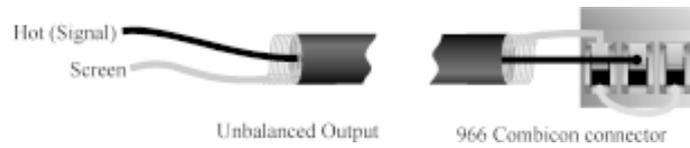
When feeding the FCS 966 **to** unbalanced sources, connect as follows. Note the link between *the two end pins*.
