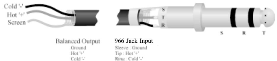
When feeding the FCS 966 from unbalanced sources, connect the signal conductor to the jack plug tip and the cable screen to the plug ring and shield.
