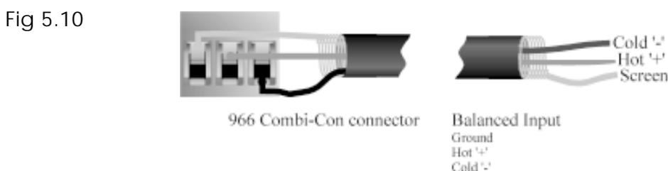
When feeding the FCS 966 **from** unbalanced sources, connect as follows. Note the link between *the two end pins*.
